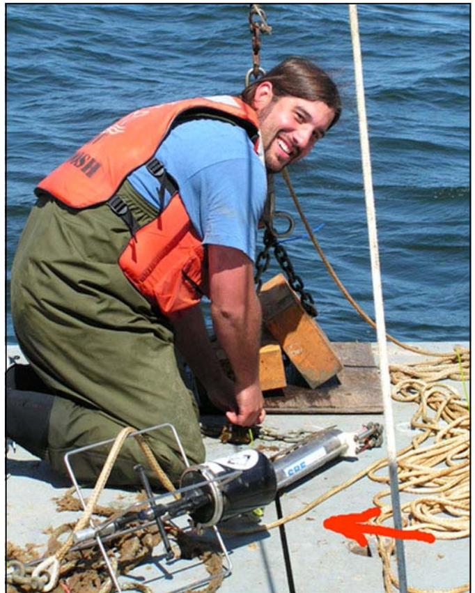
Dave Kirner is working with the current meters, in foreground, and attaching six small yellow thermistors to the line.
