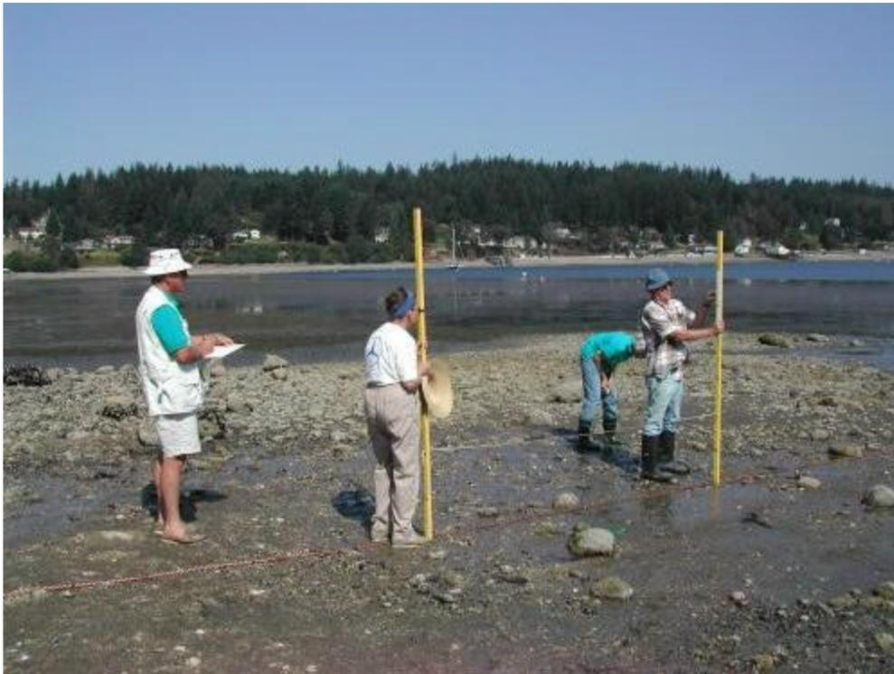
**FIGURE 4. How to Use Profile Poles (photo)**
